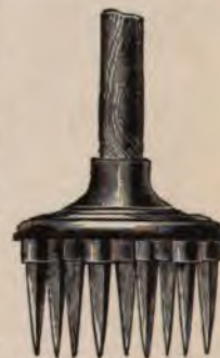
Fig. 184. Spiked ice crusher.
